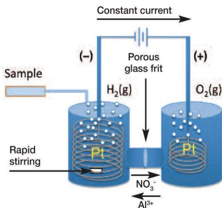
Cell for  $\text{Al}(\text{NO}_3)_3$  (aq) electrolysis.
